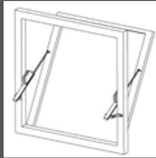
Installation on bottom hinged windows outward opening
