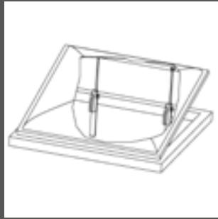
Installation on domes
