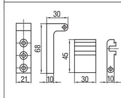
Aluminium dovetail pivoting bracket part No. 40560T
