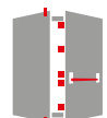
MULTIPOINT EXIT with extension for emergency or panic device + second leaf semi-fixed with espagnolette
